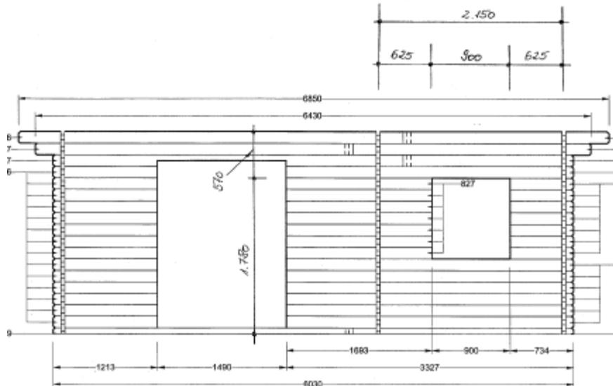
$$\begin{aligned} G &= 500 \text{ N/mm}^2 & H_u &= 1780 \text{ mm} \\ b &= 44 \text{ mm} & H_o &= 570 \text{ mm} \\ l &= 2150 \text{ mm} & l_o &= 900 \text{ mm} \end{aligned}$$
